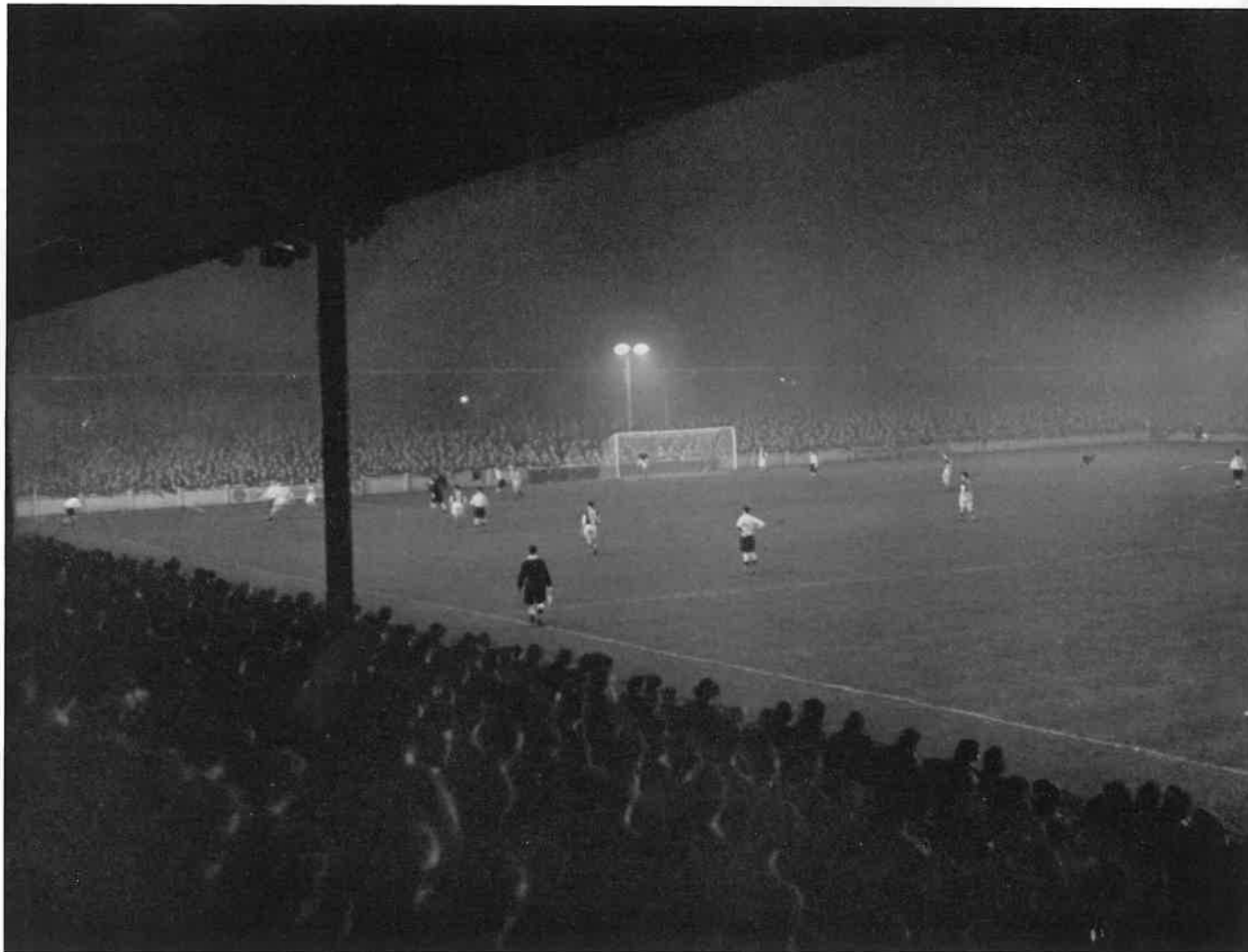
A floodlit match between Coventry City and the well-known Scottish club, Queen of the South. Coventry City installed BTH 'Touchline' floodlighting at their ground early last season. The special BTH 'Low Brightness' Football Floodlighting Projectors house 1500-watt general service tungsten lamps.
