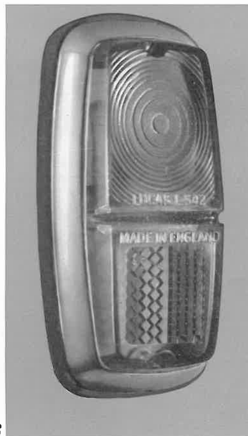
Fig. 6. A recently developed plastic stop-tail lamp incorporating a reflex reflector. Better lamp design and improved plastic moulding and colour transmission control have resulted in vastly improved side and tail lamps during the post-war period.
